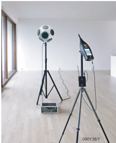
Fig. 15 Reverberation time measurements measured using the interrupted noise method
