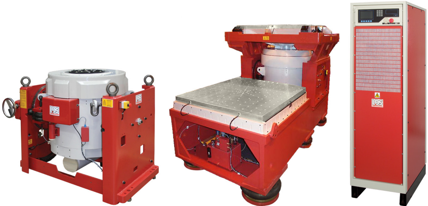
left: V8-440, trunnion-mounted with Lin-E-Air suspension; centre: combo shaker with slip table and guided head expander; right: SPA-K amplifier
