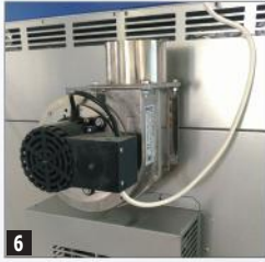
6 Air cooling extractor
