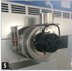
5 Air outlet extractor
