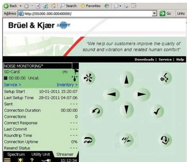
Data can be streamed over LAN-based communication or via 3G, with a maximum deviation of two seconds from the NMT to the central control server with Brüel & Kjær noise management solutions. Once on the server, Brüel & Kjær's central control software client can access and analyse the data.
