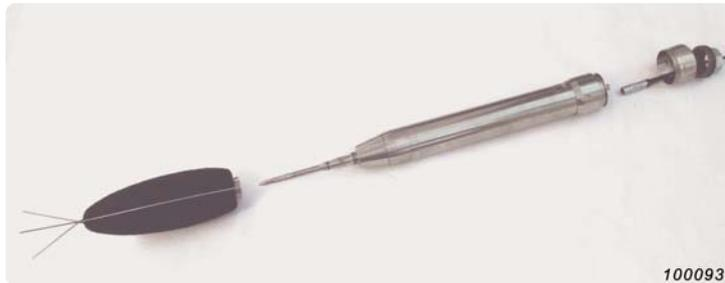
NMTs fitted with the Weatherproof Microphone Type 4184-A become suitable for specialist use where monitoring in a high-humidity or corrosive environment or where you wish to use an electrostatic actuator for remote calibration checks.
