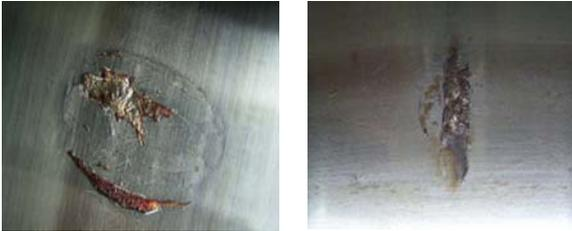
Figure 9. Damaged inner race of generator end bearing.
