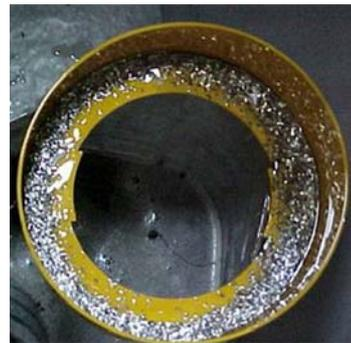
Figure 4. Oil filter of second-stage gearbox.
