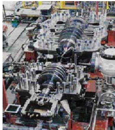
Figure 1 Typical crack gas compressor (Mitsubishi)
