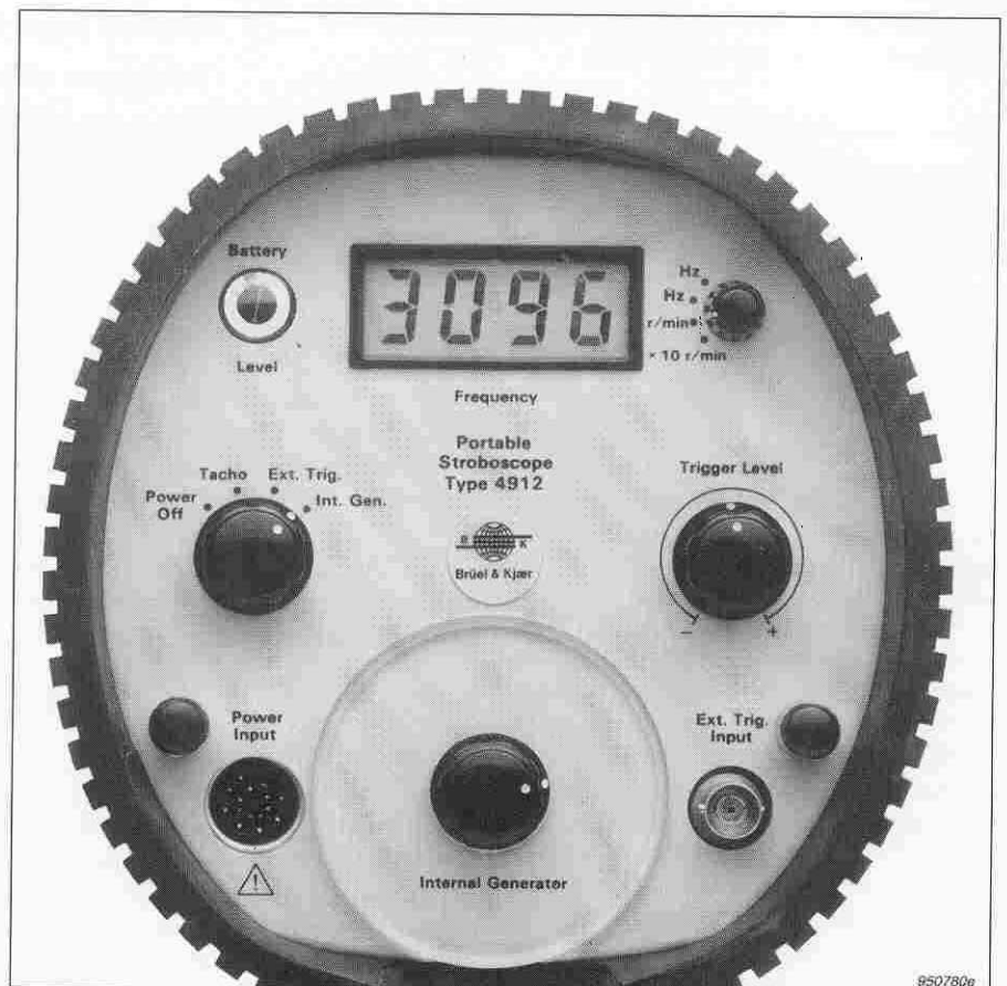
Fig.4 Control panel of Type 4912, showing Rubber Sheath DS0594 fitted for protection
