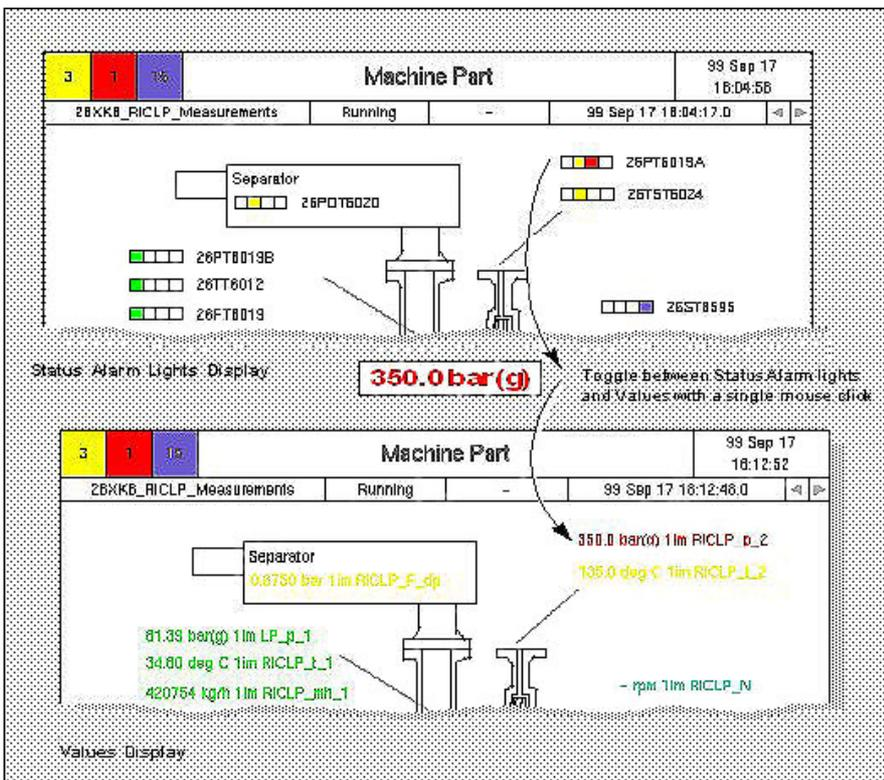
Fig. 2 Toggling between the Status 'Traffic Light' alarms and the measurement value
