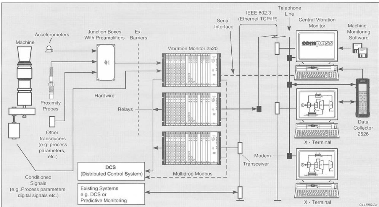
*Fig 1. The COMPASS monitoring system. Protective, predictive, performance, permanent and/or portable monitoring can all be accommodated in a single system. COMPASS can also be readily integrated to a Distributed Control System. With a choice of communication methods, plantwide system distribution or remote monitoring is no problem*
