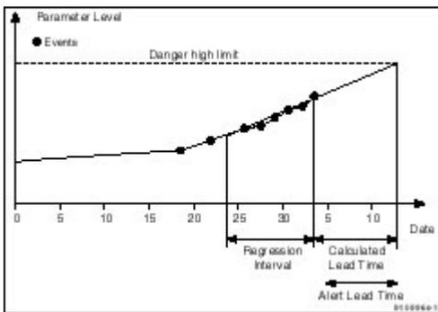
Fig. 7 Manual or automatic trend monitoring for predicting trouble
