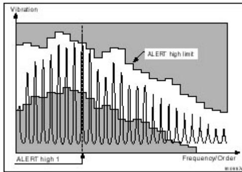
Fig. 6 Spectrum monitoring for earlier fault detection and detailed analysis
