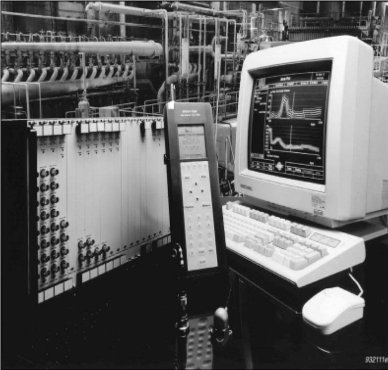
The **Type 3540 Computerized Prediction, Analysis and Safety System (COMPASS™)** provides optimized, cost effective monitoring to assure total machine protection and early recognition of faults.
