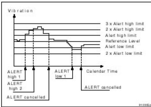
Fig. 5 Overall-level monitoring for a wide variety of safety and performance applications
