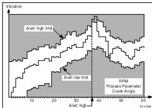
Fig. 8 Profile measurements for transient speed machinery
